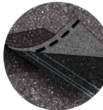
Ceramic coating Mineral core Copper layer Diagram for illustrative purposes only.
